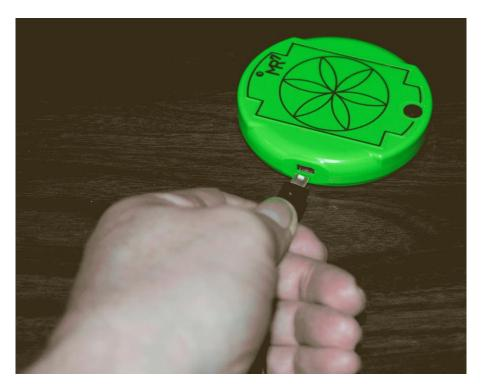
Make sure the MR7 is OFF and plug the USB cable into the MR7. The MR7 is OFF if the green LED (by the MR7 label) is not lit.
